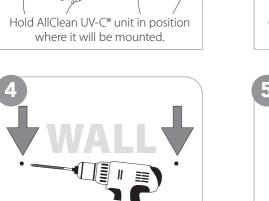
Put AllClean unit down and pre-drill holes for mounting screws.
